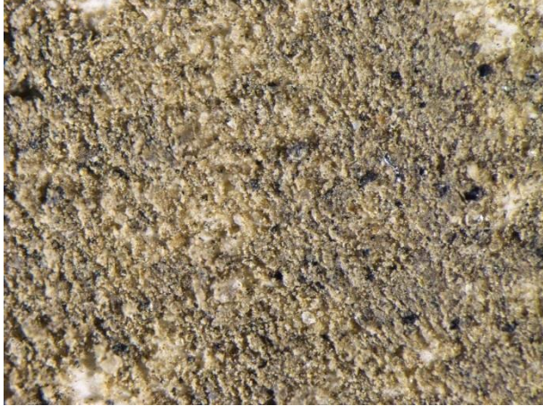
StMPM1. CV-DSI-0417, UQMP # 14907. Very small dark brown to gold coloured particles with a number of black angular particulates, typical of coal noted and dispersed through out the deposit.
