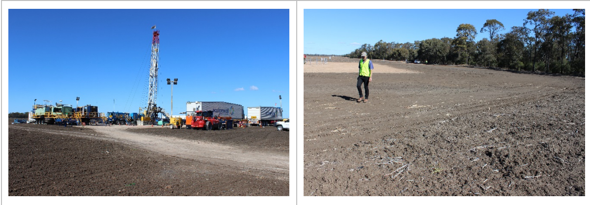
Figure 30 (left) Workover rig operating on farmland near Chinchilla, Queensland. (right) Surface soil compaction evident after operation of workover rig shown left
