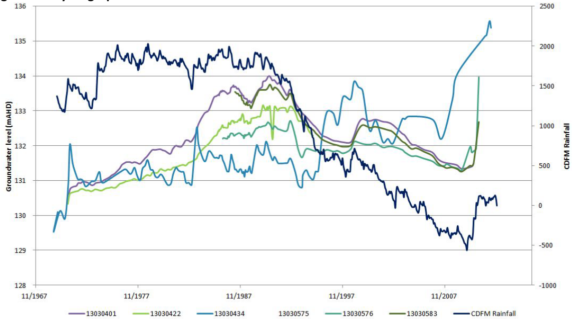
Figure 3-6 Hydrographs for selected bores installed in the Dawson River alluvium
