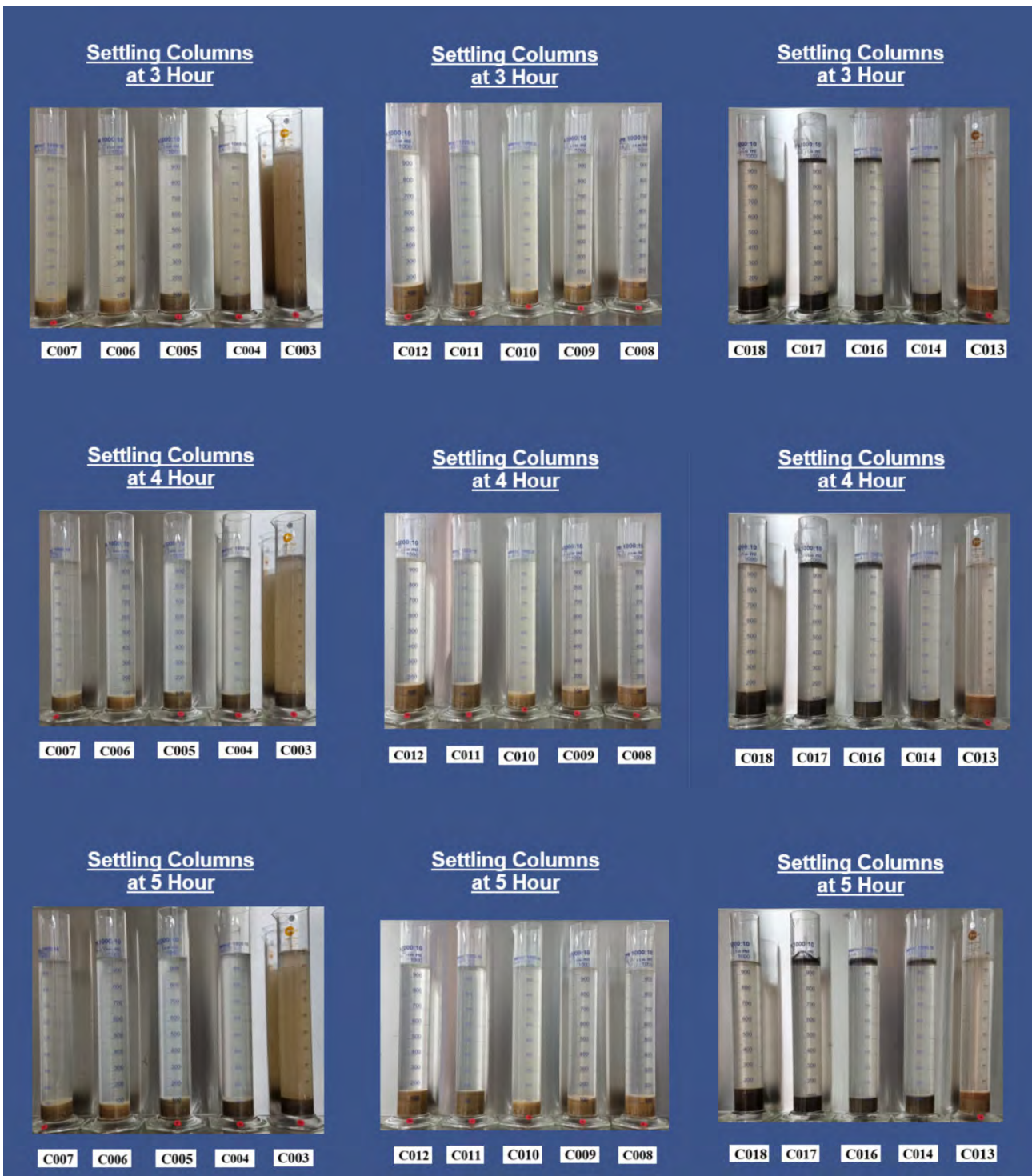
Figure 4-32: Column settlement results (3 - 5 hours)
