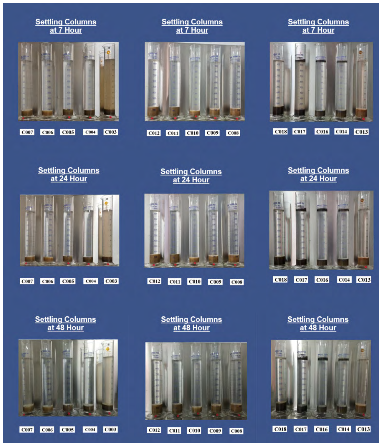
Figure 4-33: Column settlement results (7 - 48 hours)
