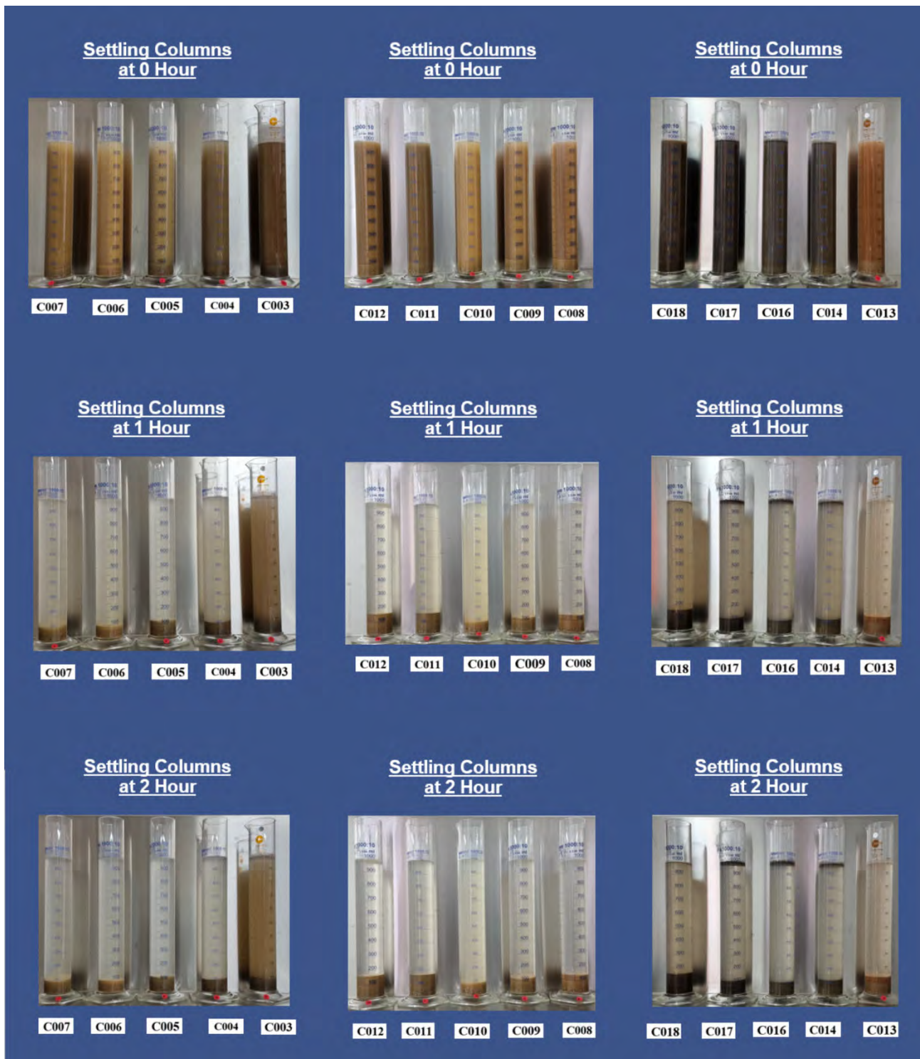
Figure 4-31: Column settlement results (0 - 2 hours)
