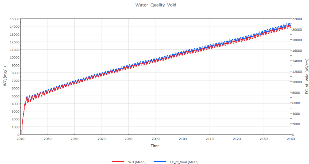
Figure 5-6: Scenario 2 – Simulated EC of the Final Void (median results)
