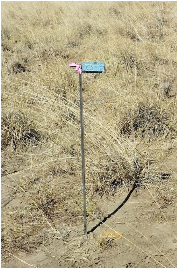
Photo 1. Camera set-up showing vertical orientation during the April survey
