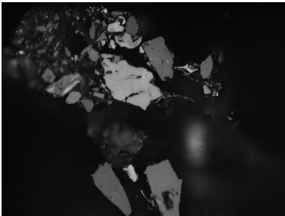
Figure 1: (CV-TIS4-0119), Coal dust particles, with the darker grey Vitrinite and lighter grey/white of Inertinite; 50x objective, oil immersion, reflected white light.
