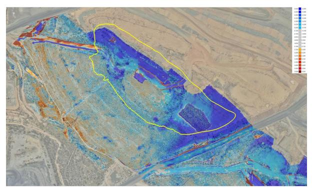
Figure 8: Johnson Pit Landform settling between June 2018 and Sept 2021
