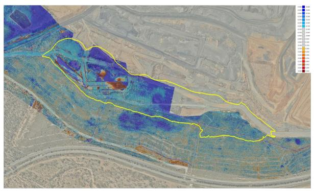
Figure 7: South Pit Landform settling between June 2018 and Sept 2021
