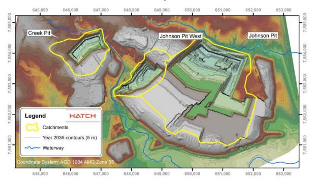
Figure 9: 2016 Study Final Landform and catchments considered for Void Water Balance Model
