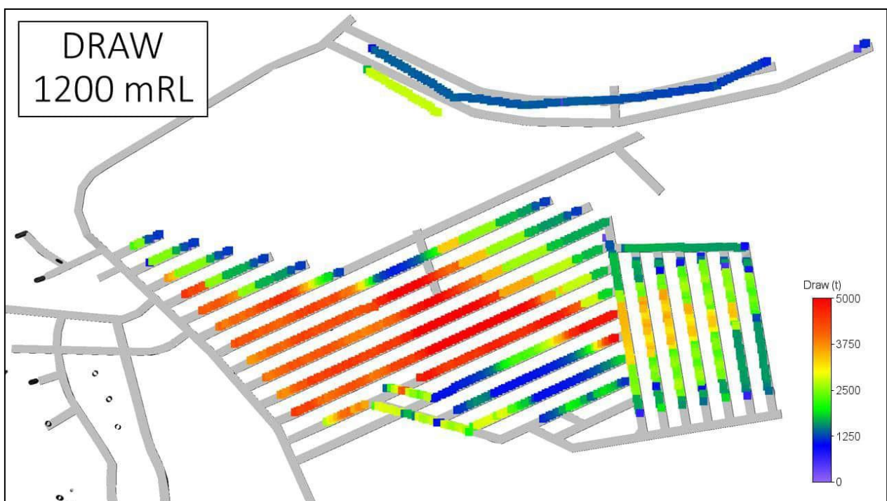
Figure 2-16 Example of simulated production draw for one sublevel of the SLC (top view, 1200 Level).
