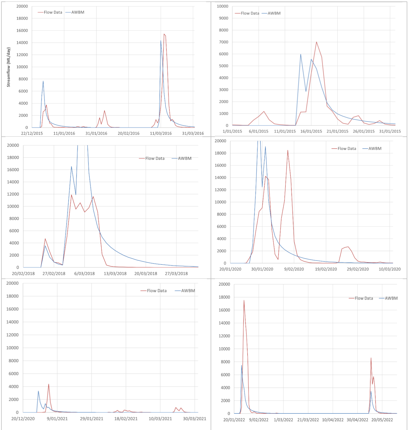
Figure 6.4: Saxby River AWBM Calibration Result – Daily Flow for Individual Events
