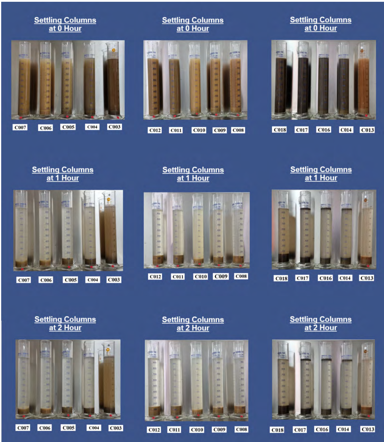
Figure 4-31: Column settlement results (0 - 2 hours)
