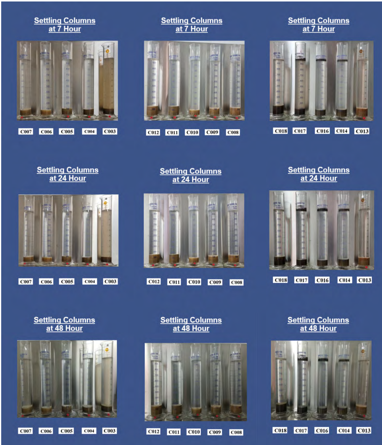
Figure 4-33: Column settlement results (7 - 48 hours)
