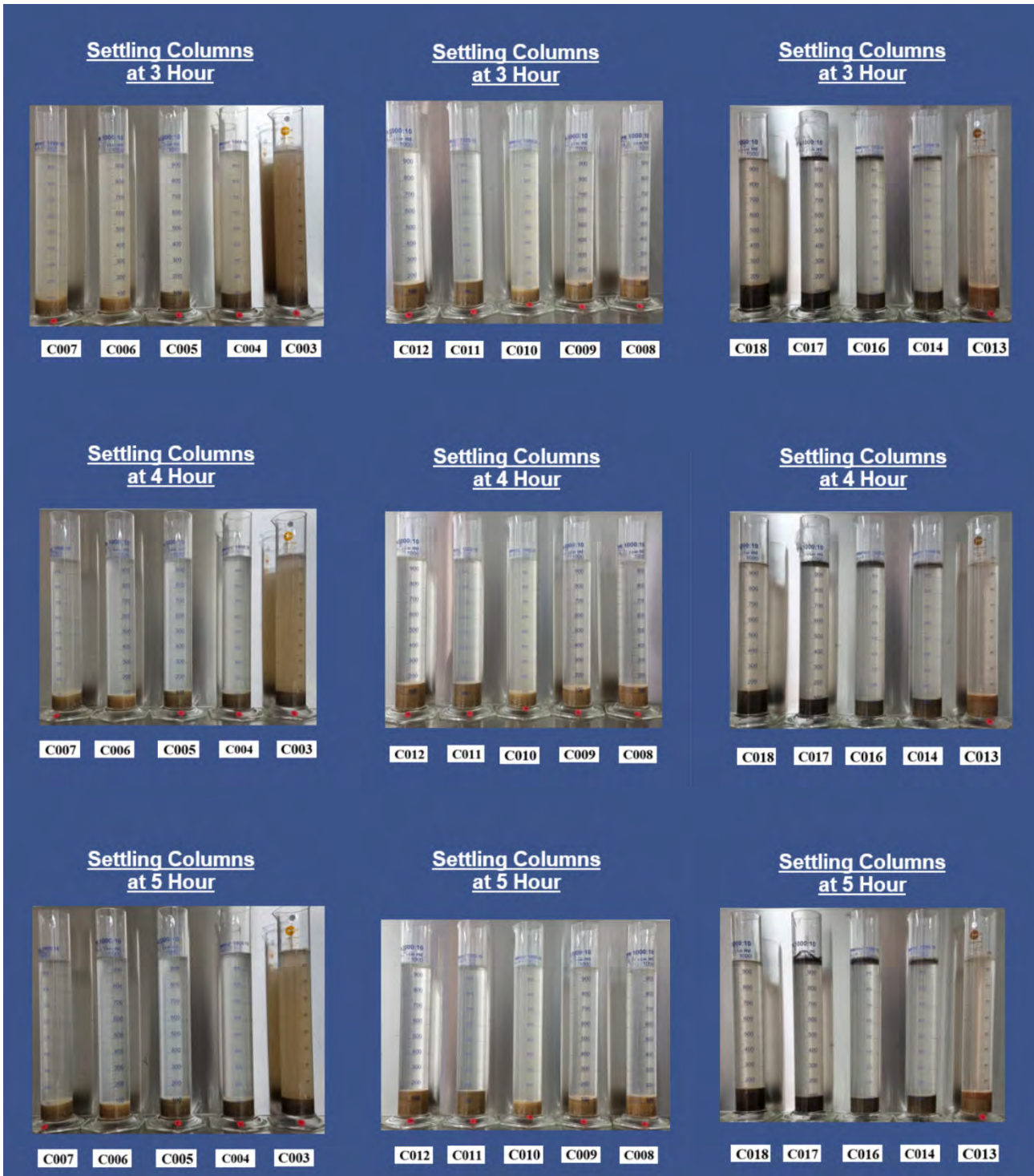
Figure 4-32: Column settlement results (3 - 5 hours)
