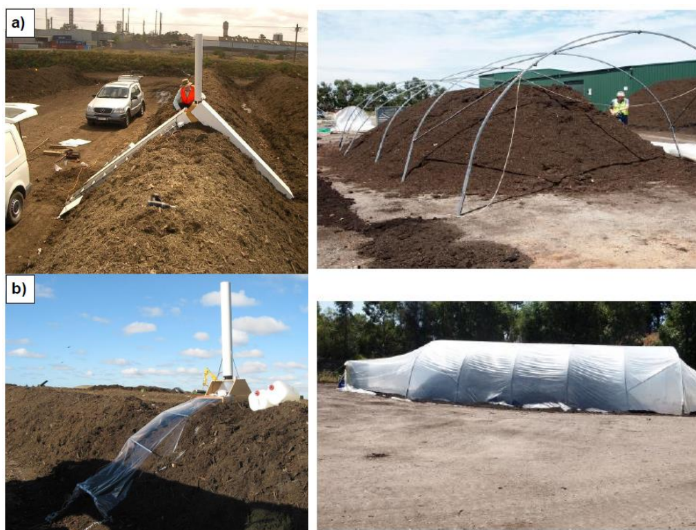
Figure 6: Sampling compost stockpiles using versions of the Draped Wind Tunnel (upper and lower left) and a Full Enclosure 'Greenhouse' method (upper and lower right) (Pollock and Braun, 2009 and Pollock et al. , 2015)
