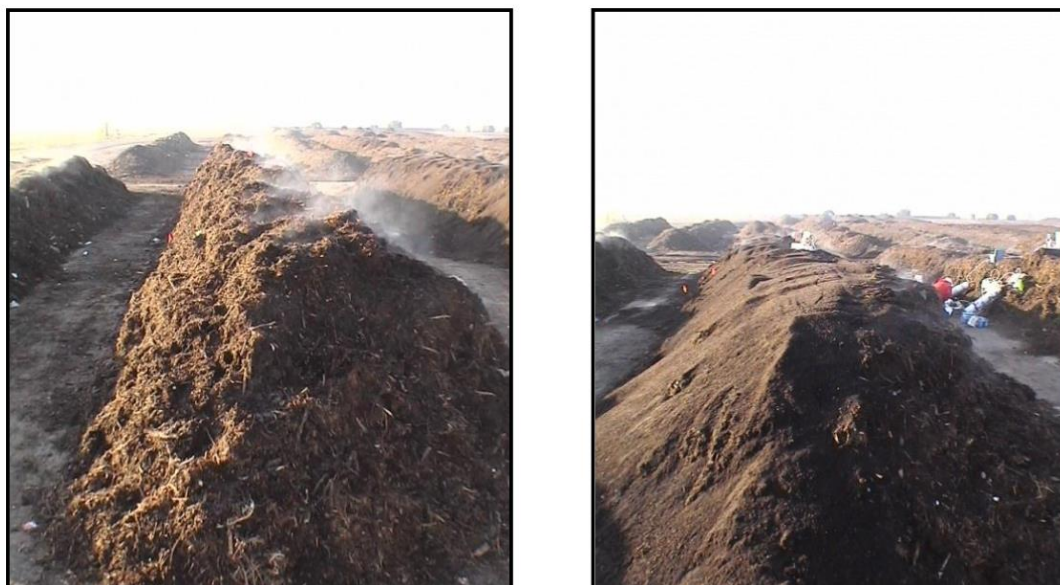
Figure 19 Visual comparison of emissions from an uncapped windrow (LHS) versus a capped windrow (RHS) from California (Buyuksonmez, 2011)
