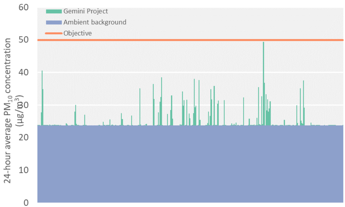
Figure 21 Year 8 – Timeseries of 24-hour average PM 10 at SR16 including additional mitigation (when required)
