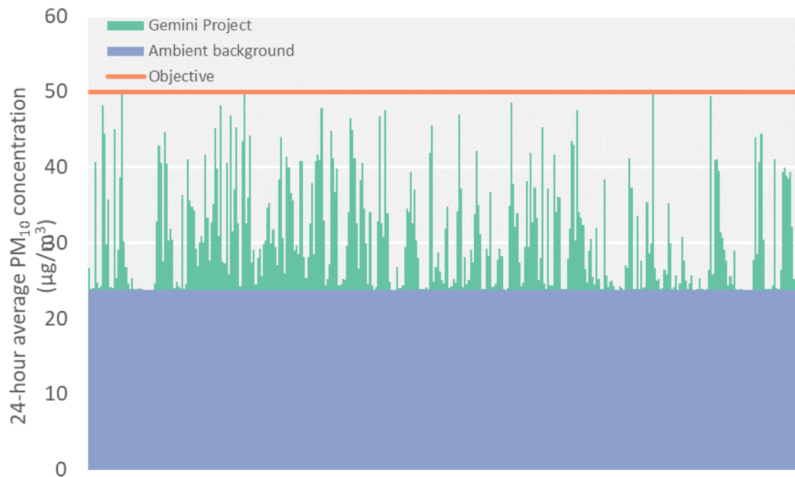
Figure 32 Year 15 – Timeseries of 24-hour average PM 10 at SR32 including additional mitigation (when required)
