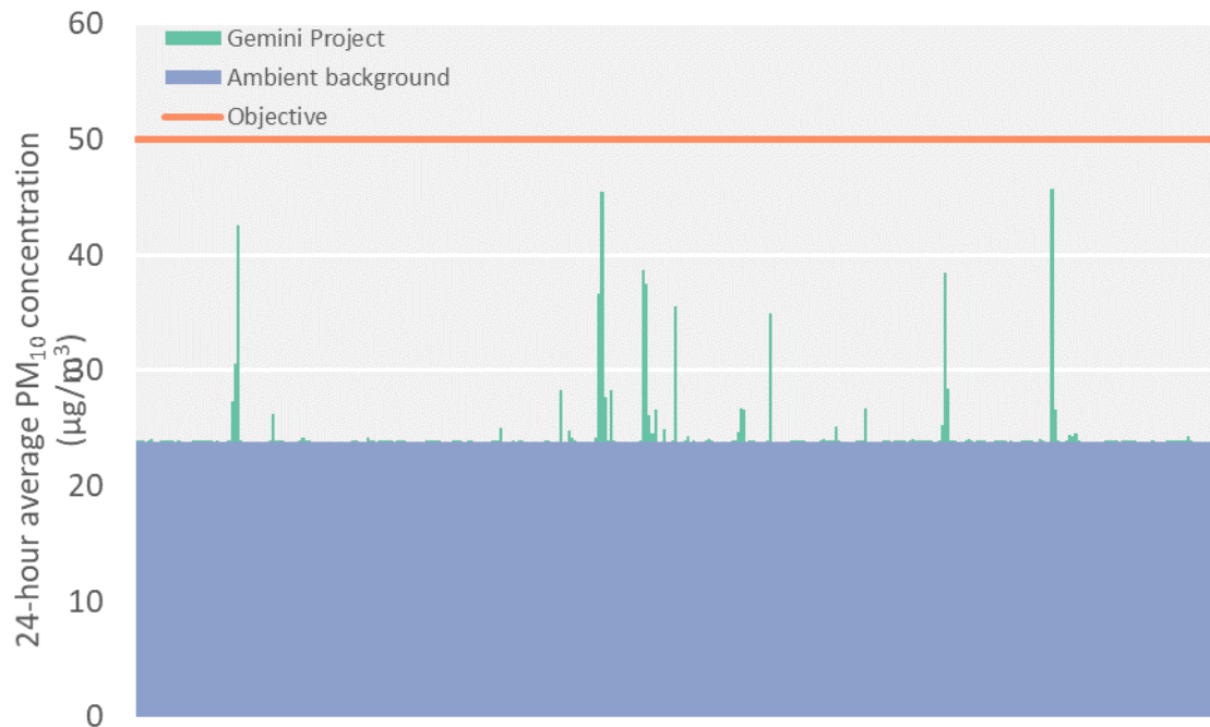
Figure 23 Year 8 – Timeseries of 24-hour average PM 10 at SR26 including additional mitigation (when required)
