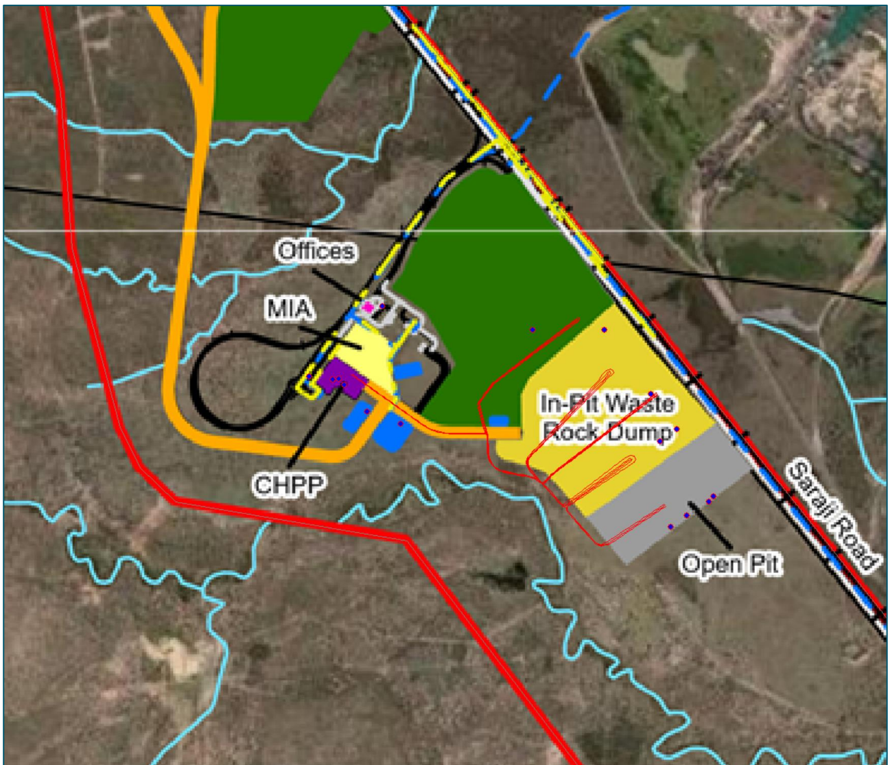
Figure D.2 Year 4 Equipment Locations in Noise Model (Note: Equipment shown as blue dots and truck paths shown as red lines)
